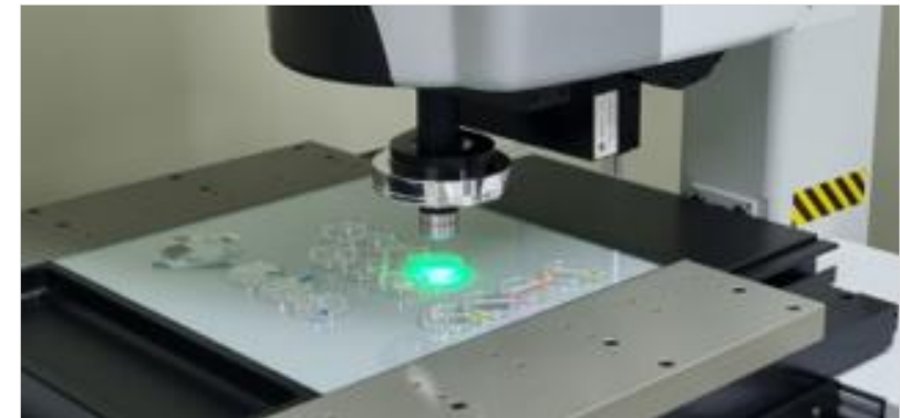
Solder Ball Dimension Auto Inspection
